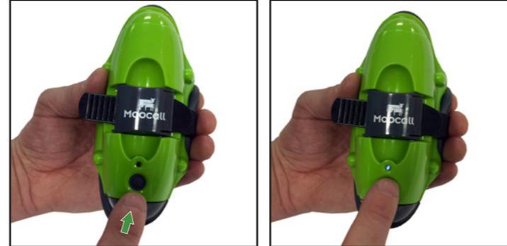
Do not turn unit off after calving (software updates are sent automatically over the GSM network and the sensor needs to be left powered on to receive same), only turn off the unit when storing for long periods.
